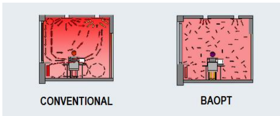
Figure 49: Conventional ventilation system and the Baopt ventilation system.
