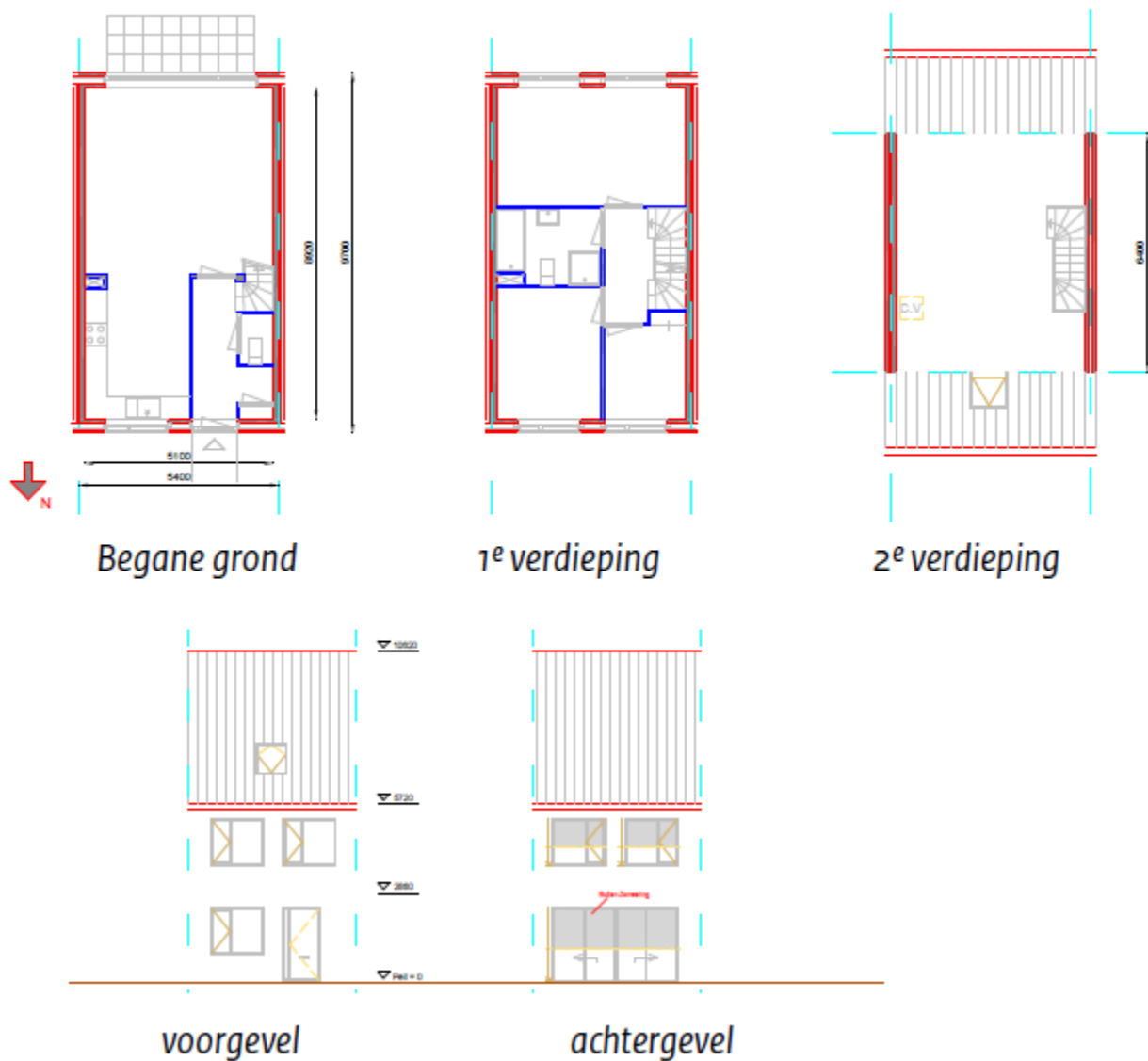
Figure 35: Geometry in-between-building terraced house. [90]
